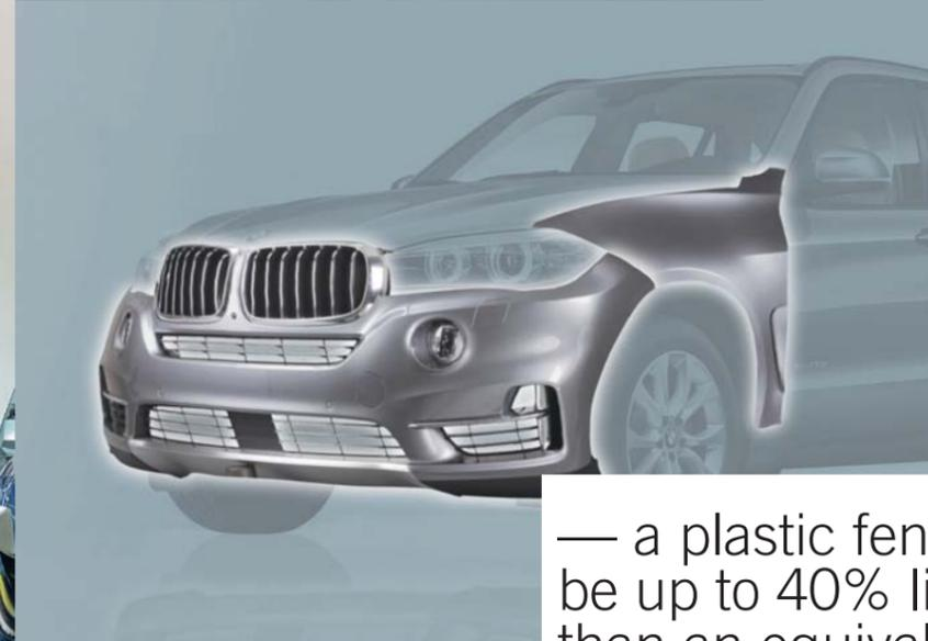
— a plastic fender can be up to 40% lighter than an equivalent metal system
