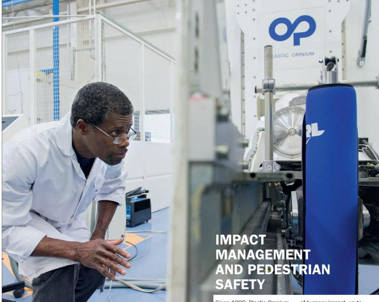
PREPARING A 40-KM/H "LEG" IMPACT TEST.
