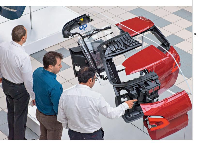
POTENTIAL TO INTEGRATE TAILGATE MODULE FUNCTIONS IN PLASTIC.
