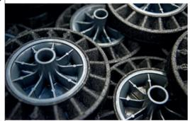
WHEELS OF ROLLING BINS PRODUCED FROM TIRE GRANULES.
