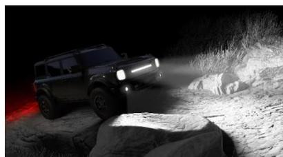
Using individually controlled LEDs, the Intelligent Off-Road Lighting System predicts illumination needs and creates a precise beam that diffuses the right light, in the right place, at the right time. This system integrates and processes vehicle data, such as the vehicle's acceleration, direction and GPS information, to seamlessly adapt the light and best illuminate the chosen path.
