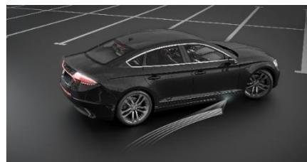
This way, the technology enhances safety and allows a sophisticated light staging. In addition to illuminating the vehicle's entrance, the module can project warning symbols in front of the driver and passenger doors, such as a snowflake in case of ice on the road.
